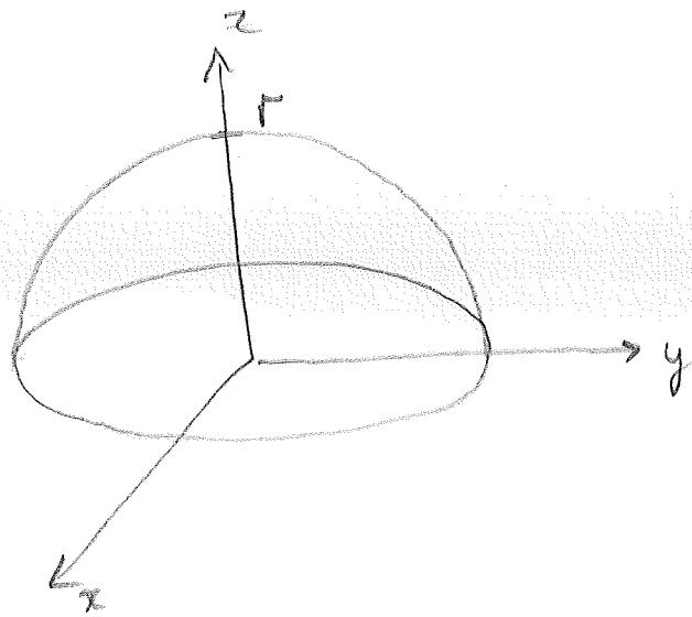
If we place the hemisphere as shown, then by symmetry  $\bar{x} = \bar{y} = 0$ , so we only need to find  $\bar{z}$ .
