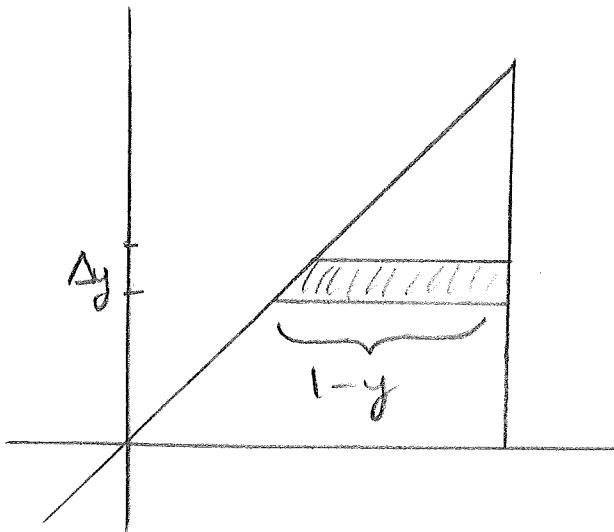
$$\begin{aligned}\delta(y) &= \sigma \times \text{length of small strip} \\&\approx \sigma(1-y)\end{aligned}$$
