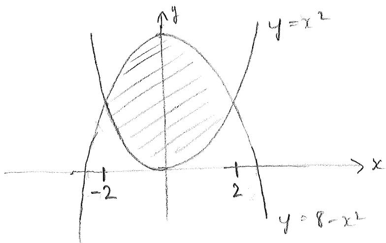
Need to intersect the curves to determine the limits of the integration in  $x$ .
