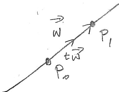
Note: A parametric representation gives us not only a path (L or S) but also a specific motion along the path.
