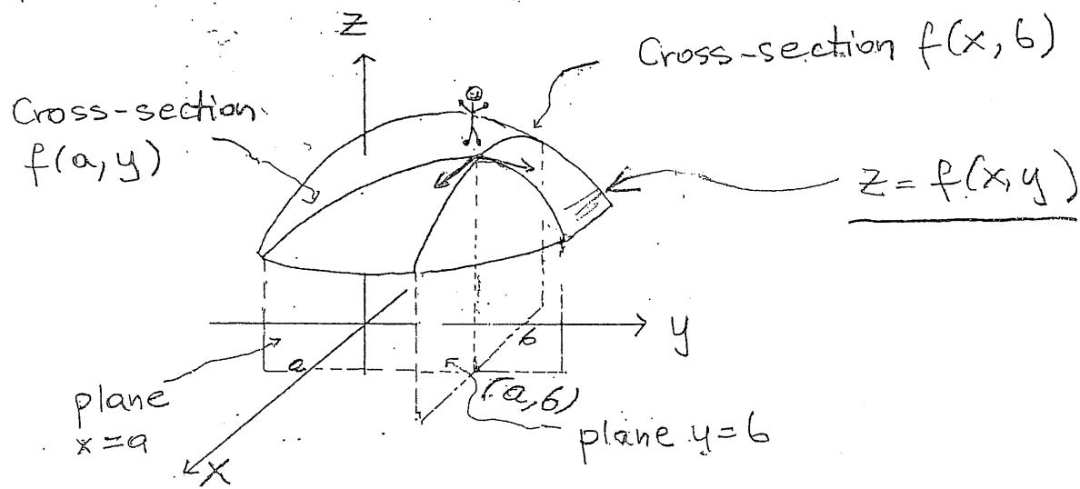
$$f_x(a, b) = \frac{d}{dx} \Big|_{x=a} [f(x, b)] = \lim_{\Delta x \rightarrow 0} \frac{f(a + \Delta x, b) - f(a, b)}{\Delta x}$$
