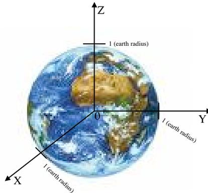
We will also assume that any point at sea level satisfies  $x^2 + y^2 + z^2 = 1$ . Time will be measured in milliseconds, (one thousandth of a second,  $10^{-3}$ ) and the speed of light constant  $c \approx 0.047$  earth radii per millisecond.
