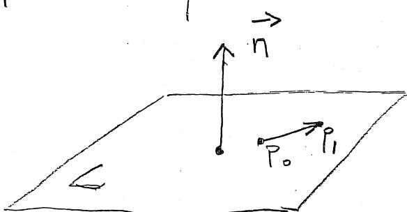
Remark: If  $\vec{n} = a\vec{i} + b\vec{j} + c\vec{k}$  is normal to a plane  $L$ ,  $P_0 = (x_0, y_0, z_0)$  is a point on  $L$ , then the equation of  $L$  is:
