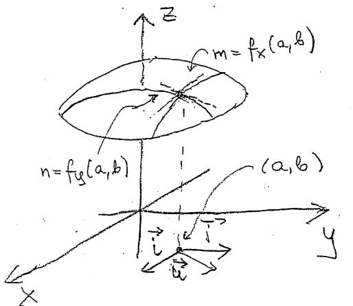
$f_x(a, b)$  gives us the rate of change when we walk from  $(a, b)$  in the direction of  $\vec{i}$ ,  $f_y(a, b)$  if we walk in the direction of  $\vec{j}$ .
