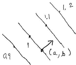
You obtain fastest growth by moving perpendicularly to contours in the direction of increasing values. So  $\nabla f(a,b)$  that points toward fastest increase must be perpendicular to contours.
